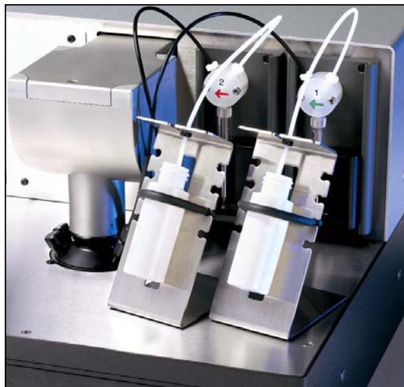
Figure 3. Close up of two injector syringes and reagent bottles. Clarity can be provided with up to 4 syringe injectors. Note that each injector has a freely movable reagent bottle holder, inert tubing and a dedicated syringe to control injection volume.
